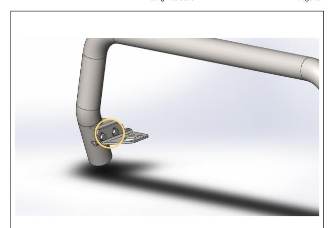
10. Loosely fit mount brackets to nudge bar with M10x25 Hex bolts, washers and flange nuts.
