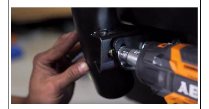
14. Position the nudge bar, if you have forward parking sensors you will need to pivot the top of the nudge bar back as far as possible towards the Jeep, and lift it as high as it will go. Then torque down bolts.
