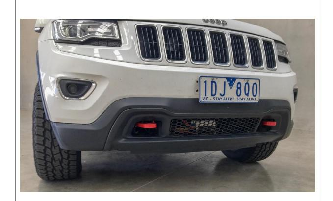
9. Refit lower skid and air dam with factory hardware.
