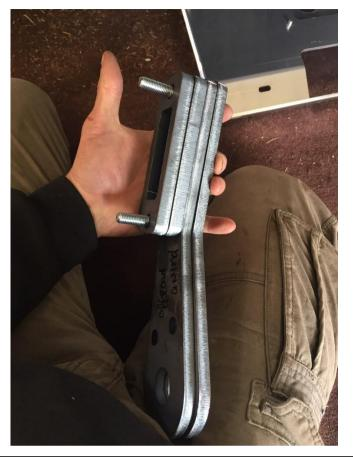
5. Stack Offroad Animal Tow points together as shown with M10 bolts and M10 flat washers.
