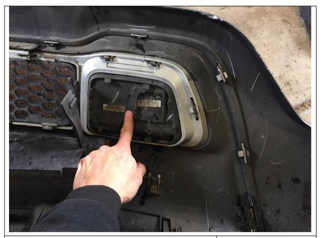
7. Locate clearance windows as shown in lower air dam.
